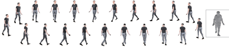
Fig. 10. Bullet-time effect rendering result. We show 21 samples out of the the 144 views in our bullet-time rendering sequence. We also show a visual hull reconstruction from the view sequence.
