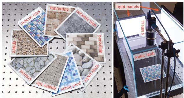
Figure 8. Our experimental setup for real data acquisition. Left: Sample reference patterns that we use for the real experiments; Right: We setup a camera on top of the fluid tank to capture refraction images of the reference pattern.
